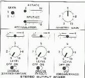
This chart provides a starting point for using the OPUS 3 owner's manual. Set all controls in this position. Note the location of the STRING, ORGAN and BRASS voice sections and the color-coding in the STEREO OUTPUT MIXER. No sound will be heard in this setting!
